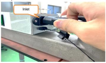
(10) Before inserting the cable, always make sure that an anti-slip cable lock is attached to the power cable as shown below.
