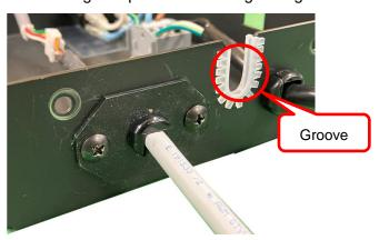
(3) Attach the cable box to the bottom of the base with four truss head screws (M4  $\times$  8 mm). (Phillips screwdriver)
